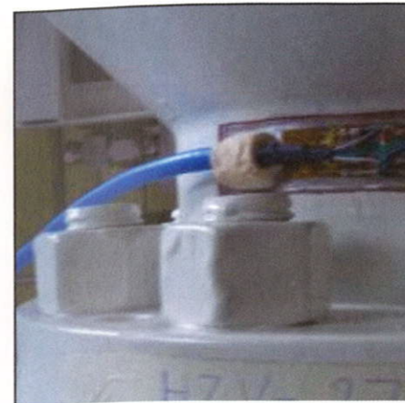
Installed Strain Gauges.
