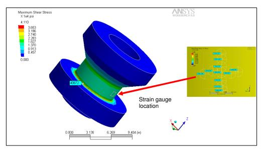
FIGURE 5 FEA of Ball Valve Mounting Stool
