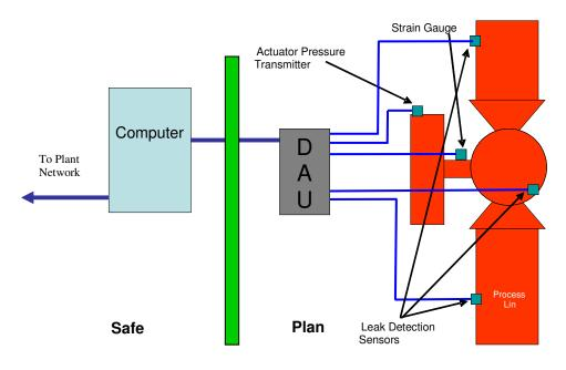
FIGURE 4 V-MAP Functional Diagram
