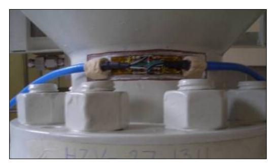
FIGURE 6 Installed Strain Gages
