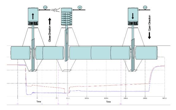
FIGURE 7 Single Acting Gate Valve Model and Example Signatures
